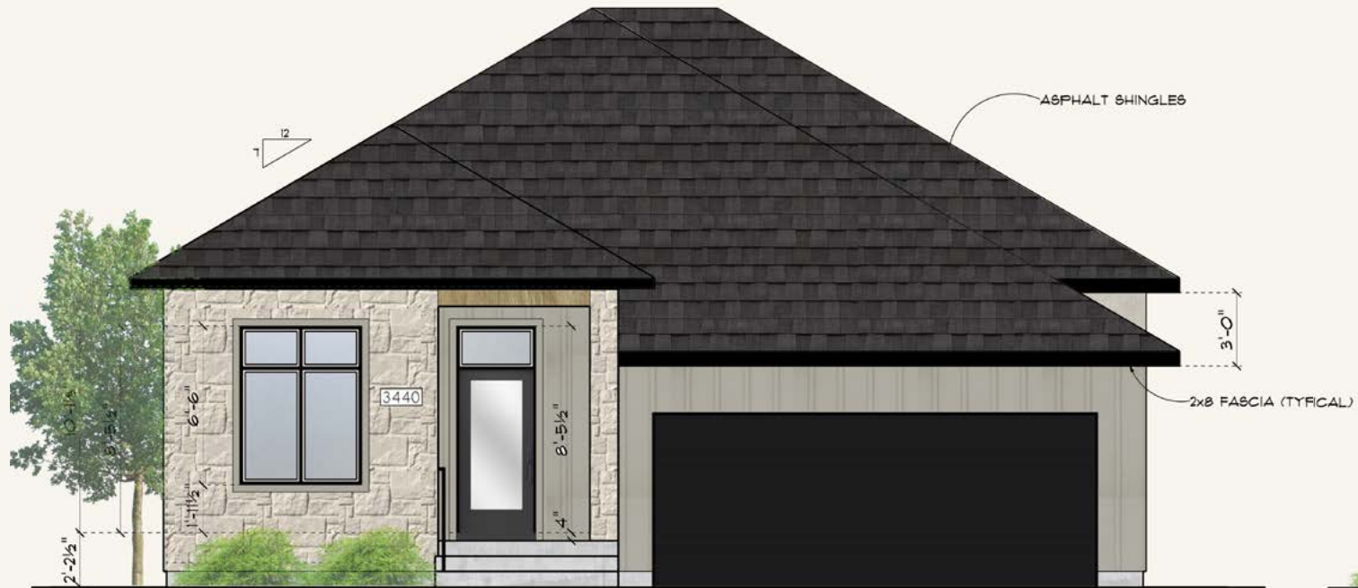
FRONT ELEVATION: NORTH
